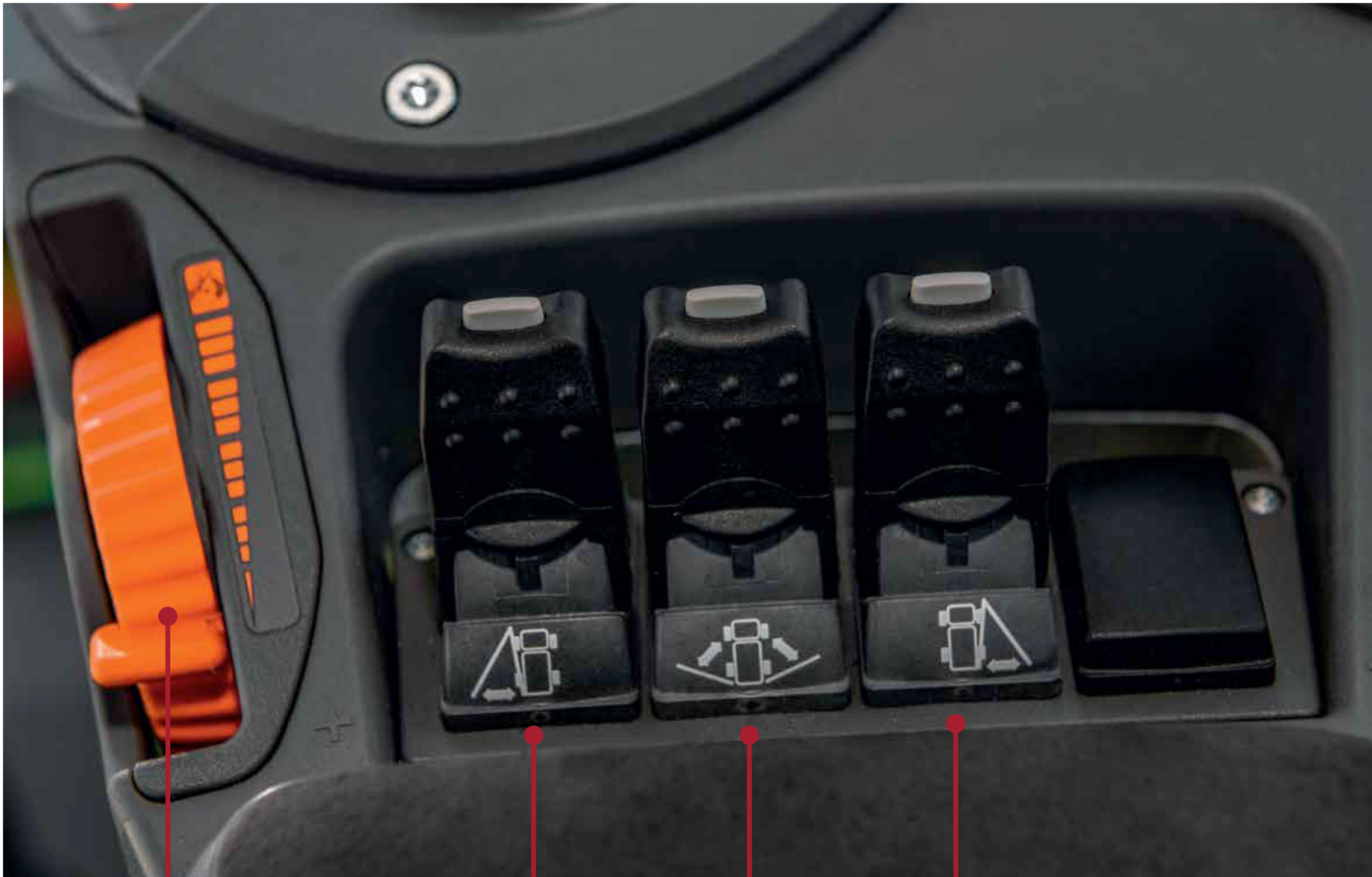
Hand throttle Folding out/folding in of the left-hand boom tip Folding out/folding in of the main boom Folding out/folding in of the right-hand boom tip
