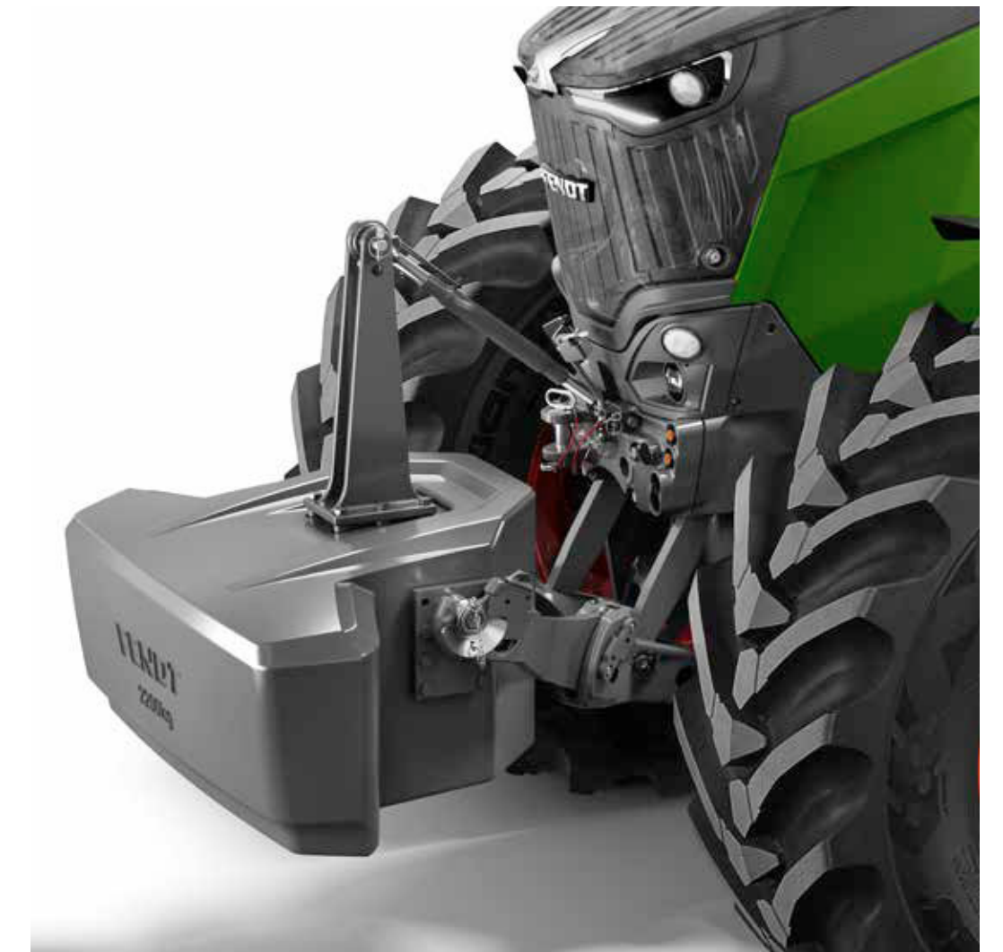
Comfort ballast support
