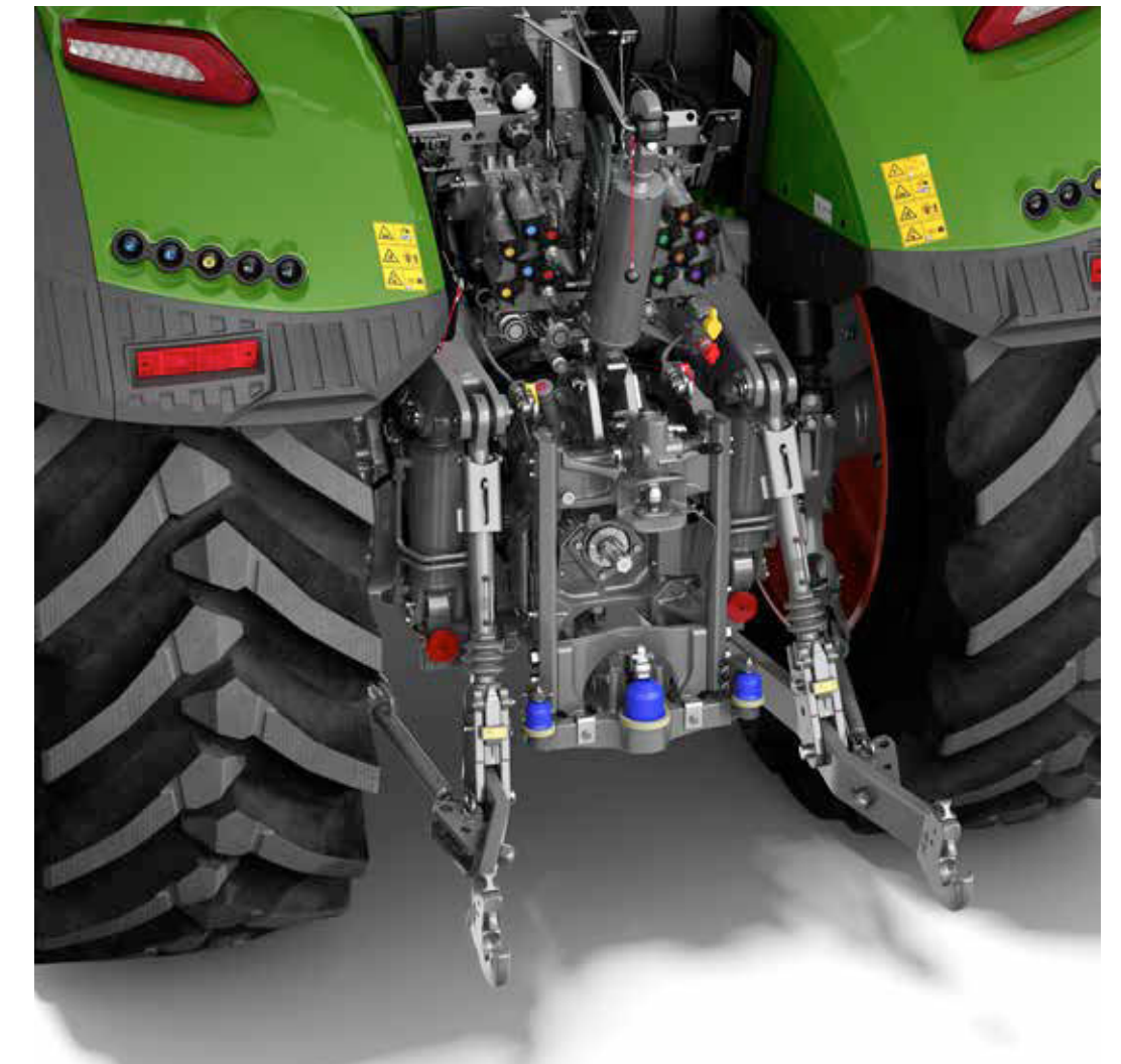
Rear power lift with quick-release hook and hydraulic side support (EU) and hydraulic top link
