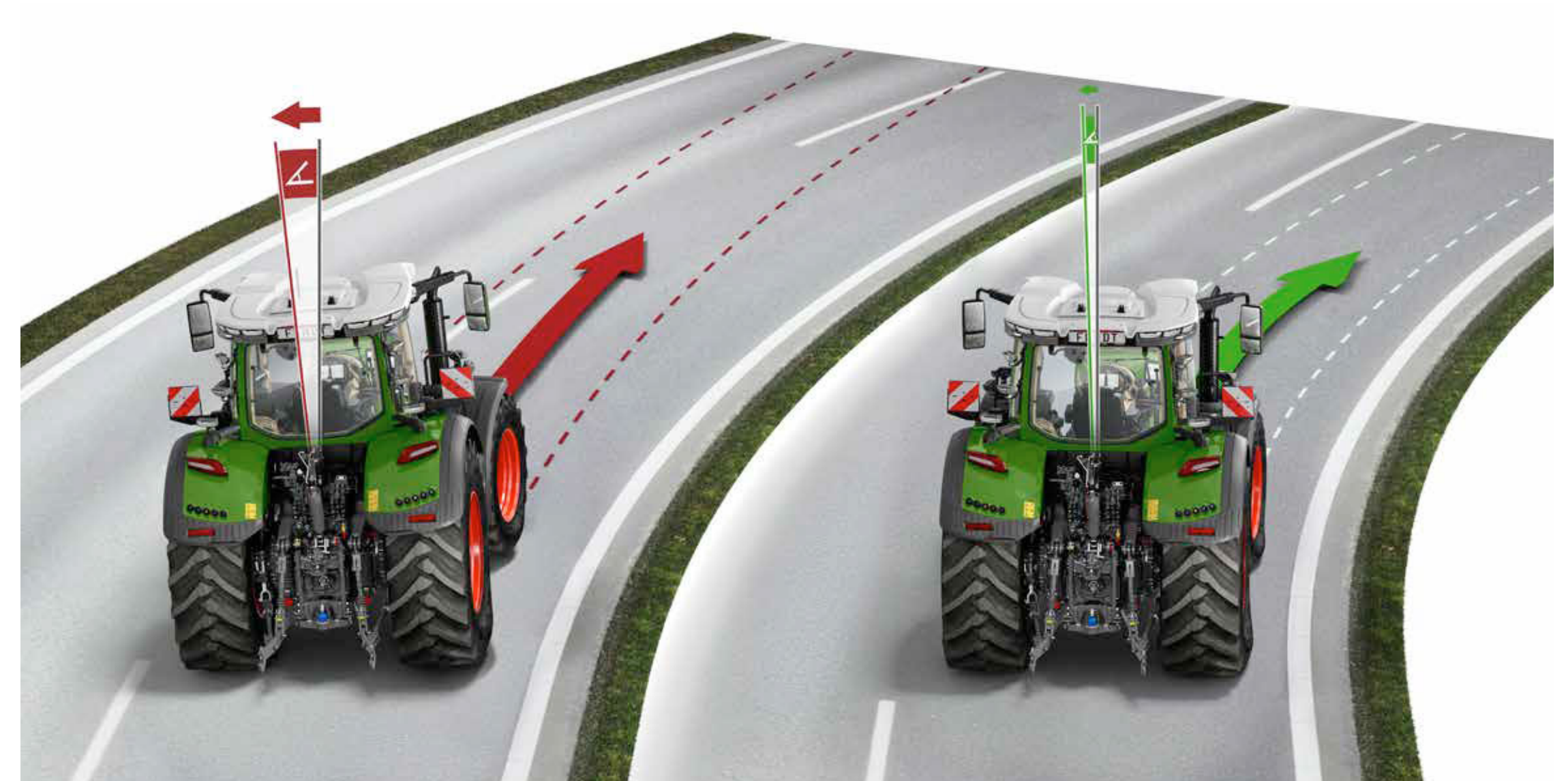
without FSC: Tractor goes off line
