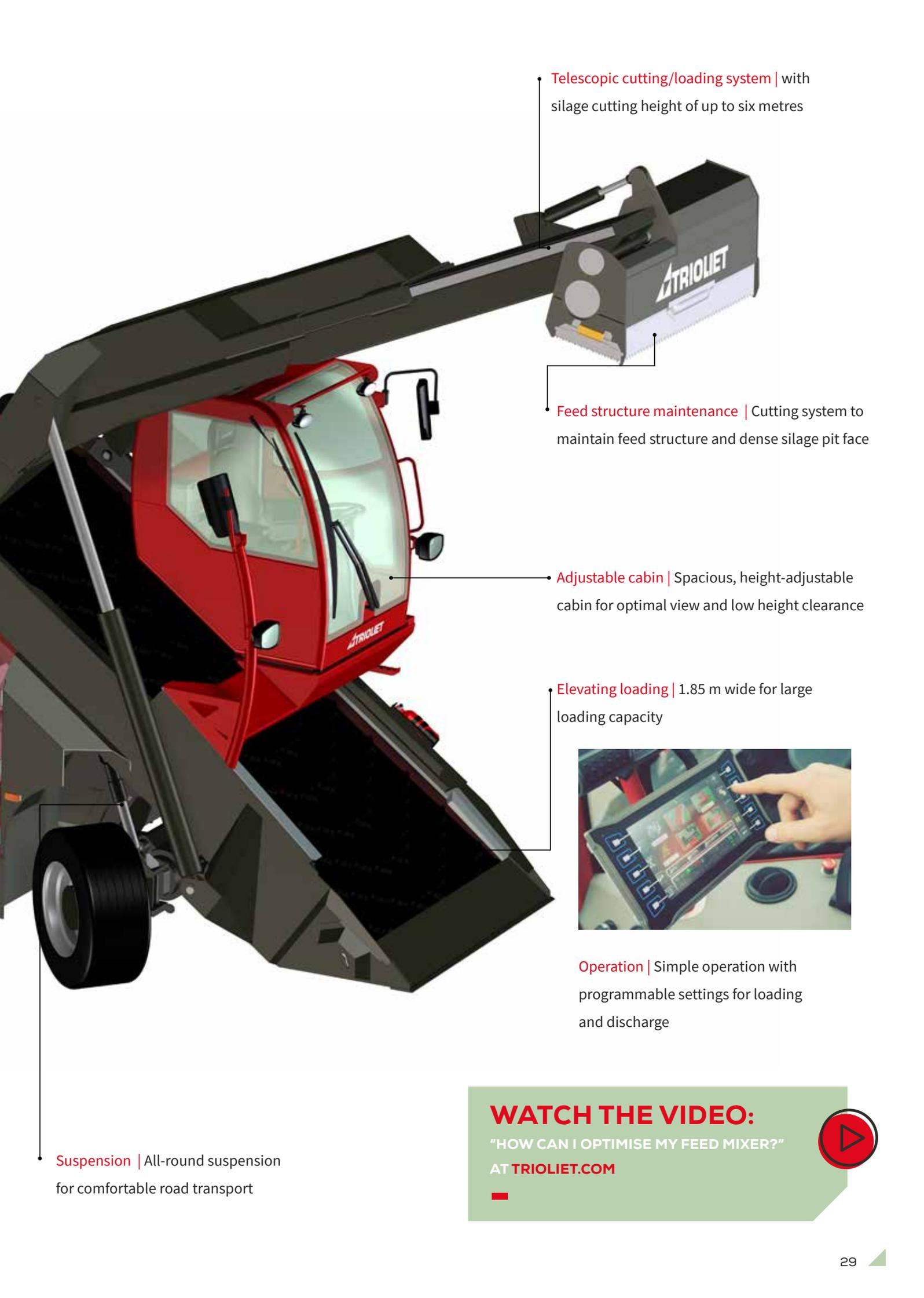
• **Telescopic cutting/loading system** | with silage cutting height of up to six metres
