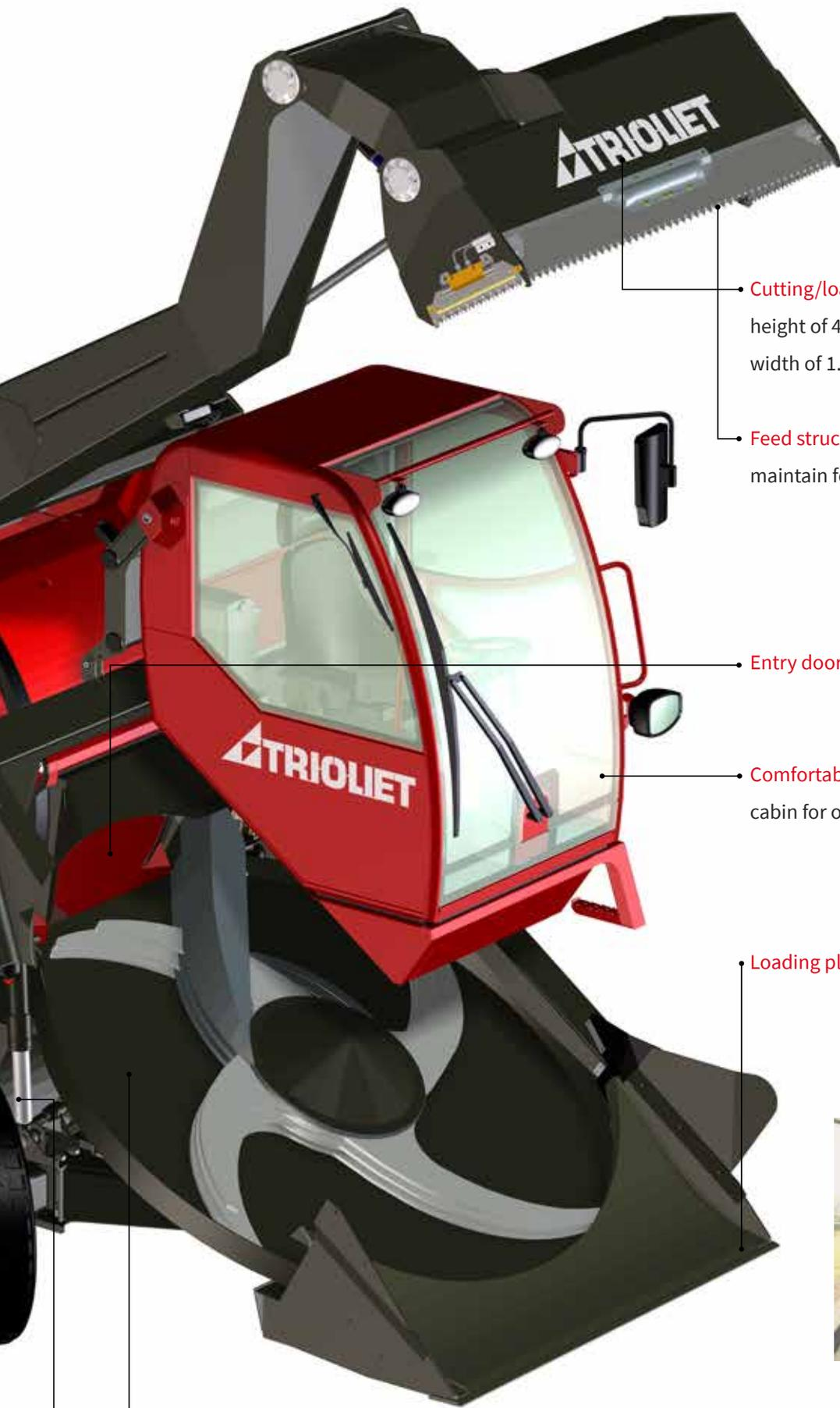
• **Cutting/loading system** | silage cutting height of 4.5 metres and silage cutting width of 1.85 metres
