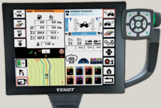
Another Spotlight is the new AdBlue consumption indicator, which not only allows you to monitor the current consumption, but also records the average and total consumption.
