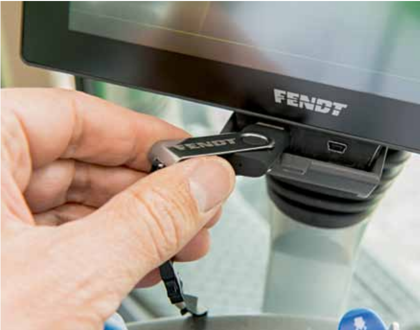
Field settings can now be conveniently exchanged amongst agricultural machinery via USB stick. Field databases are transferred via VarioDoc using Bluetooth.
